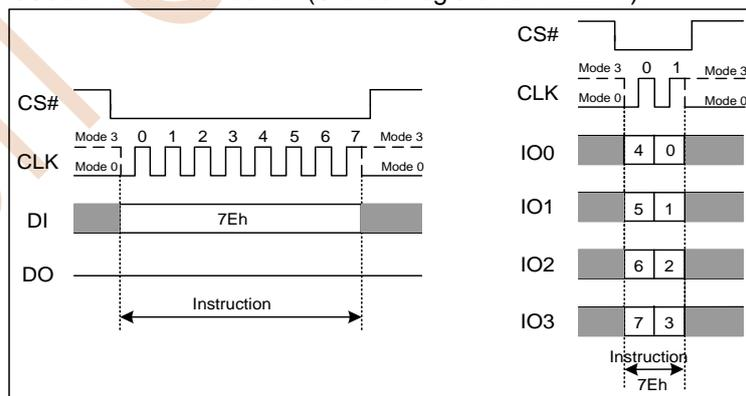
**Figure 7.39 Global Block Lock Instruction(SPI or QPI Mode)**
