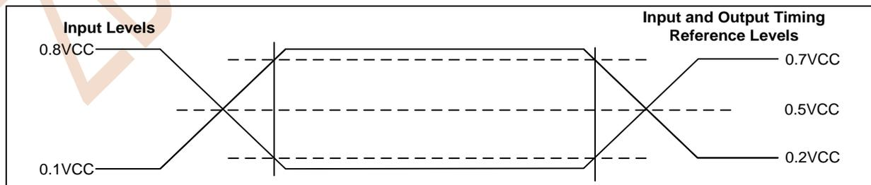
Figure 8.3 AC Measurement I/O Waveform
