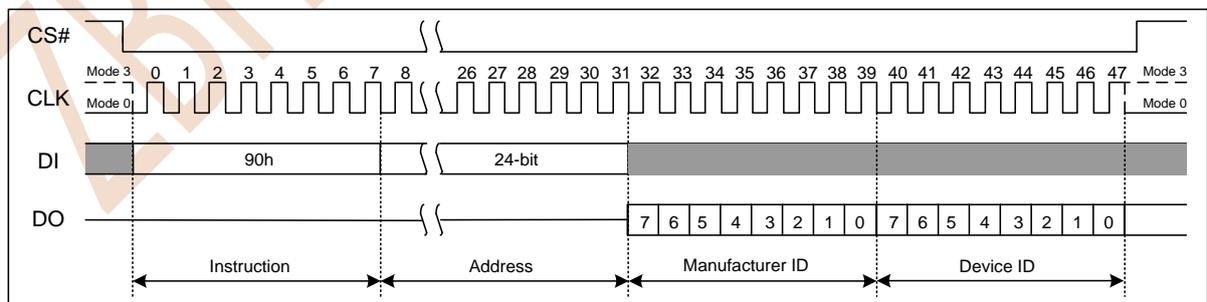
**Figure 7.30a Read Manufacturer/Device ID(SPI Mode)**
