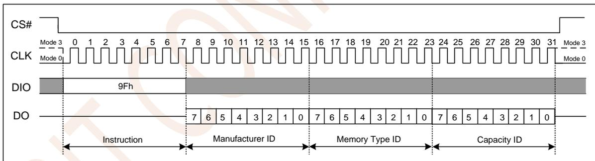
Figure 7.43a Read JEDEC ID(SPI Mode)
