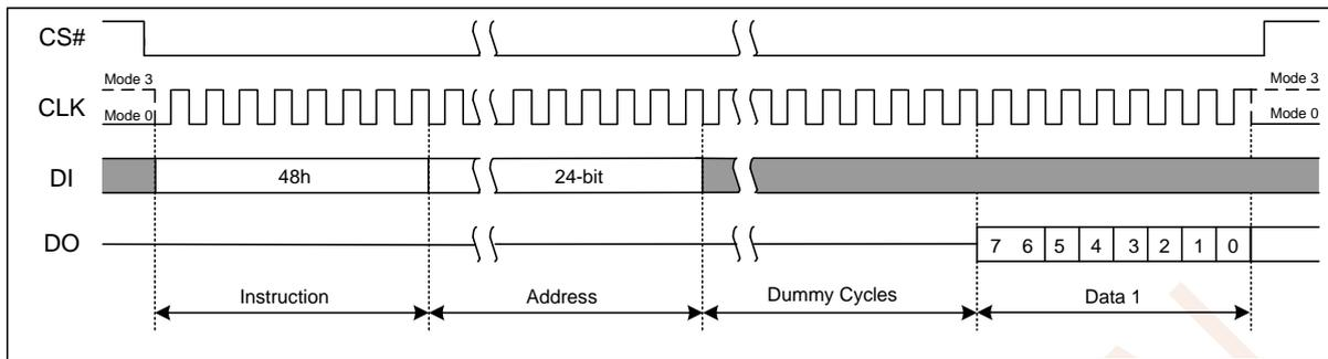
Figure 7.47 Read Security Registers Instruction (SPI Mode only)
