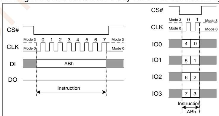
Figure 7.41a Release Power-down Instruction(SPI and QPI Mode)
