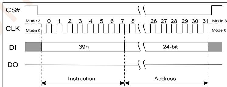
Figure 7.49a Individual Block/Sector Unlock Instruction(SPI Mode)
