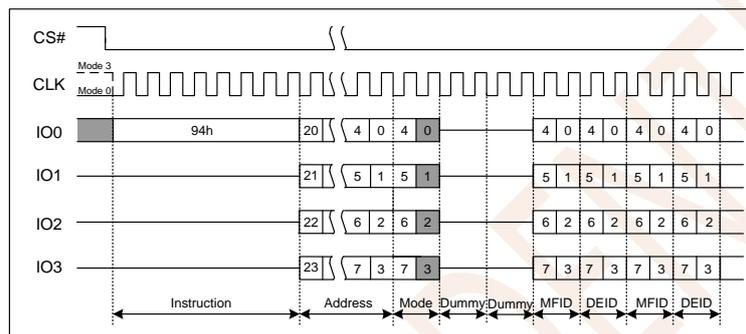
Figure 7.54 Read Manufacturer/Device ID Quad I/O Instruction
