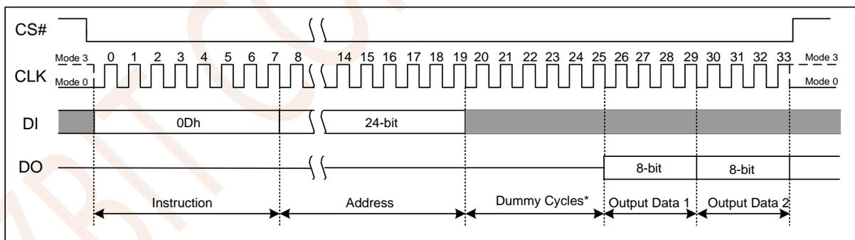
Figure 7.24a DTR Fast Read Instruction (SPI Mode)
