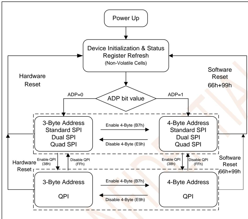
Figure 6.2 ZB25Q256A Serial Flash Memory Operation Diagram
