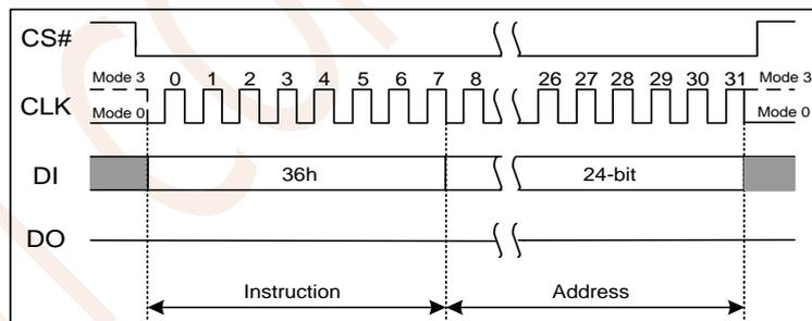
Figure 7.48a Individual Block/Sector Lock Instruction(SPI Mode)
