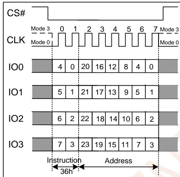
Figure 7.48b Individual Block/Sector Lock Instruction(QPI Mode)
