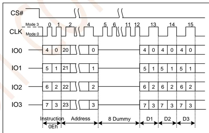
**Figure 7.58 DTR Burst Read with Wrap Instruction (QPI Mode only)**
