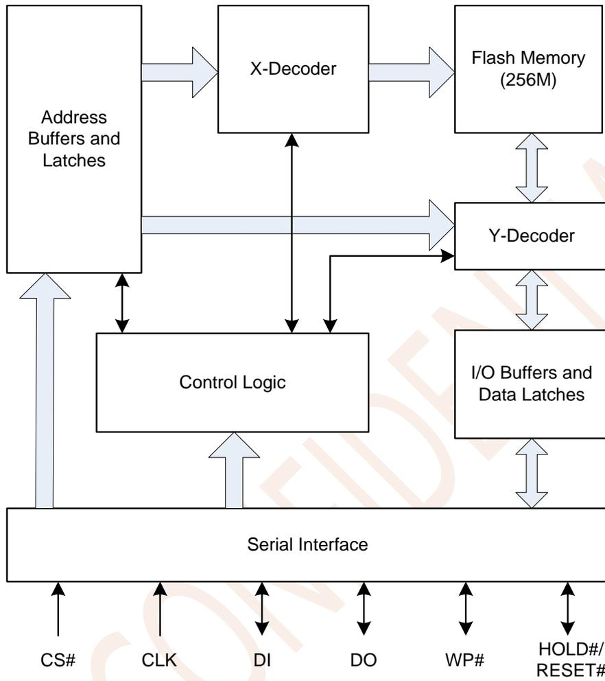
Figure 2.1 Block Diagram
