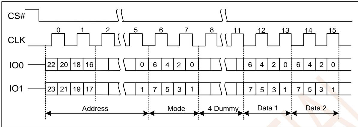
Figure 7.31b DTR Fast Read Dual I/O Instruction (Previous M5-4=10, SPI Mode only)
