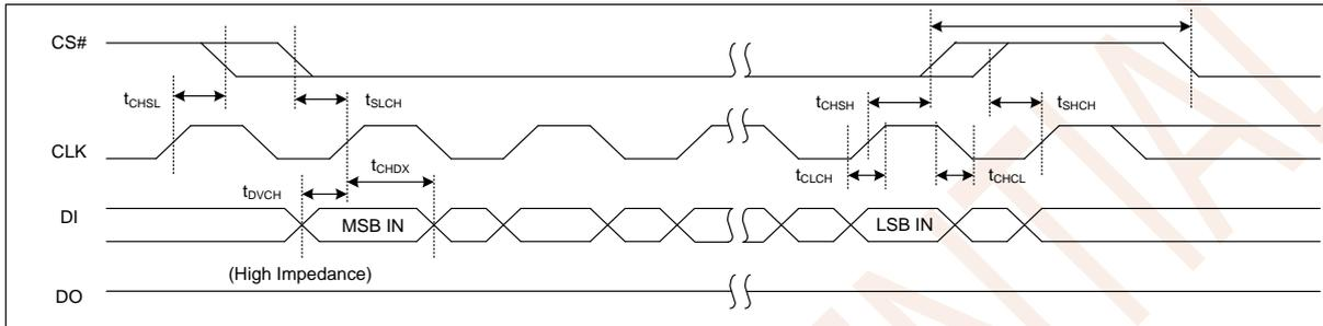
Figure 8.5 Input Timing
