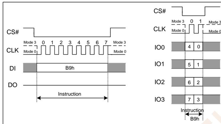
Figure 7.40 Deep Power-down Instruction(SPI and QPI Mode)
