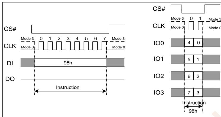
Figure 7.52 Global Block Lock Instruction(SPI or QPI Mode)
