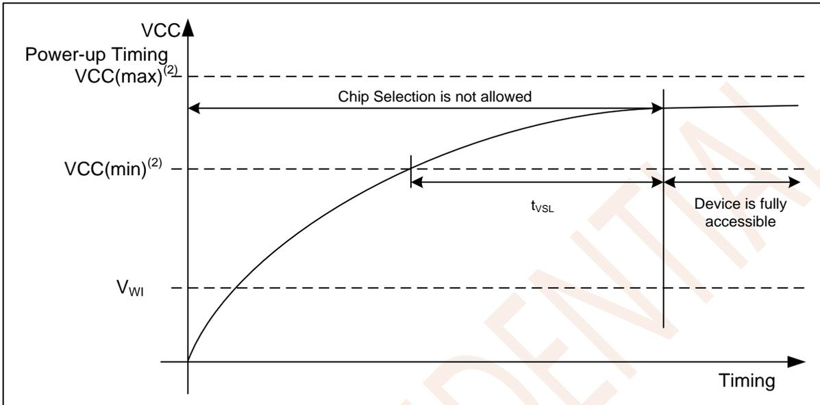
Figure 8.1 Power-up Timing
