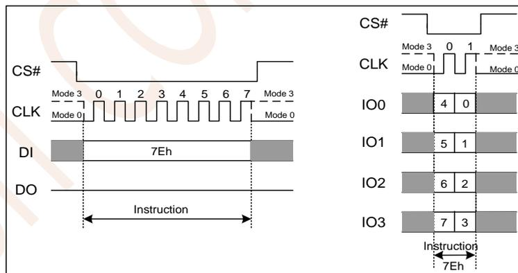
Figure 7.51 Global Block Lock Instruction(SPI or QPI Mode)
