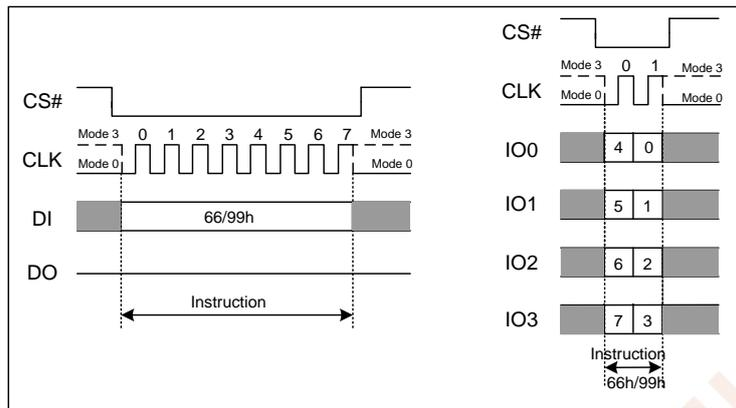
Figure 7.39 Software Reset Instruction(SPI and QPI Mode)
