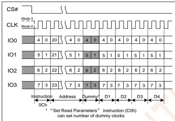
**Figure 7.57 Burst Read with Wrap Instruction (QPI Mode only)**
