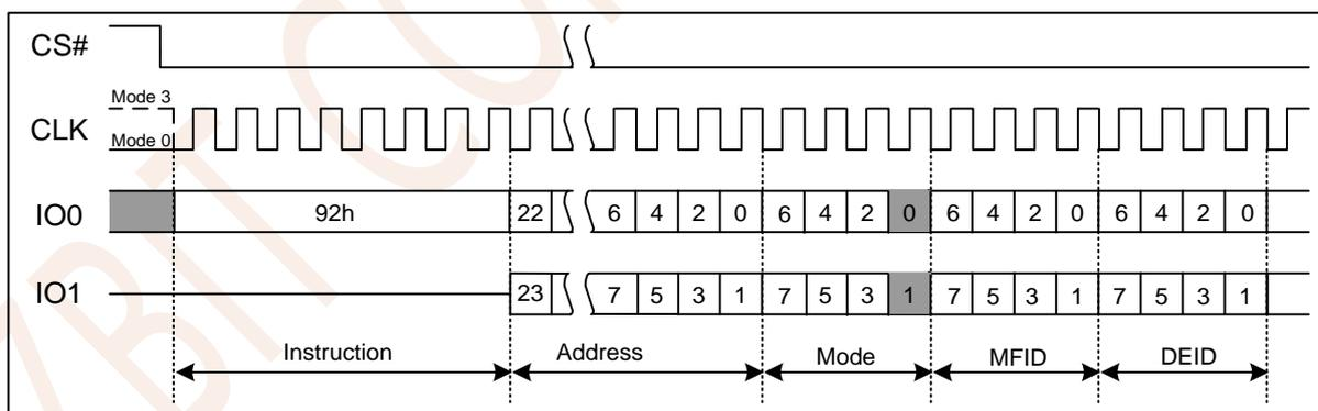
Figure 7.53 Read Manufacturer/Device ID Dual I/O Instruction
