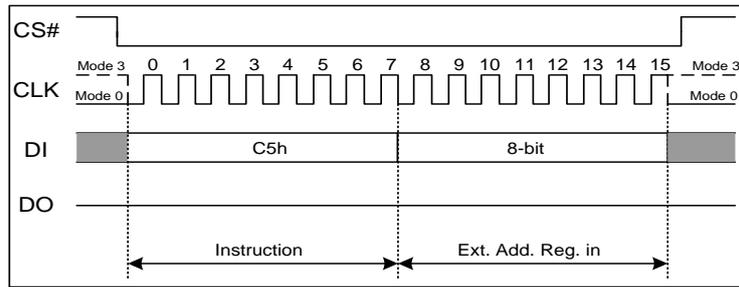
**Figure 7.7a Write Extended Address Register Instruction (SPI Mode)**
