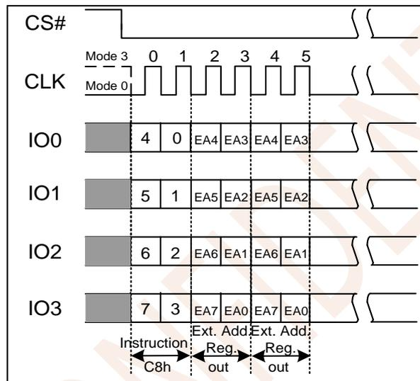
Figure 7.6b Read Extended Address Register Instruction (QPI Mode)
