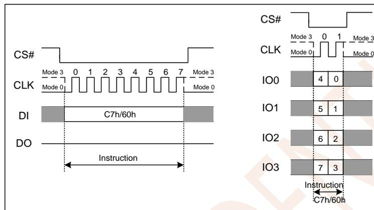
Figure 7.18 Chip Erase Instruction(SPI or QPI Mode)
