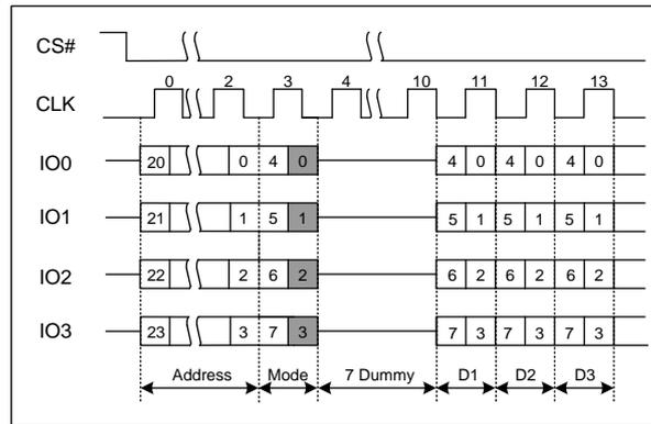
Figure 7.35b DTR Fast Read Quad I/O Instruction(Previous command set M5-4 = 10)
