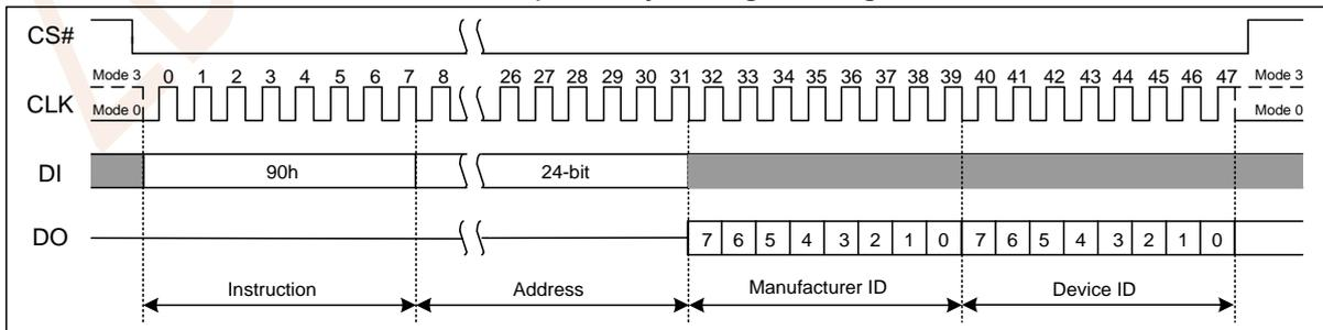
Figure 7.42a Read Manufacturer/Device ID (SPI Mode)
