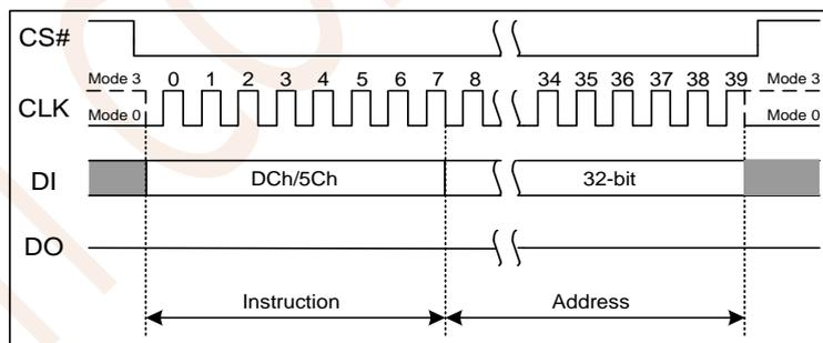
Figure 7.17 Block Erase with 4-Byte Address Instruction (SPI Mode Only)
