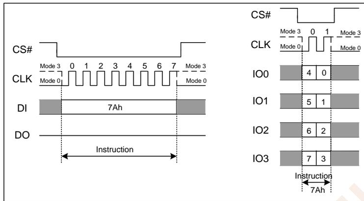
Figure 7.20 Erase/Program Resume Instruction(SPI or QPI Mode)
