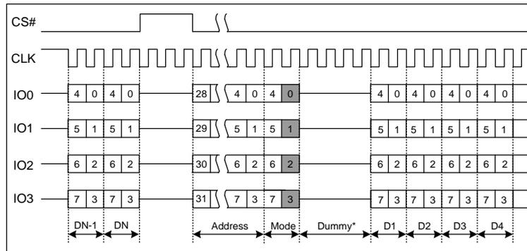
Figure 7.37b Fast Read Quad I/O with 4-Byte Address
