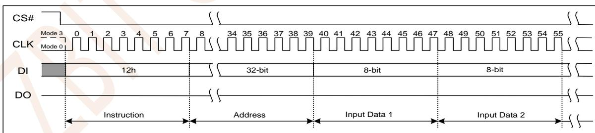
**Figure 7.11a Page Program with 4-Byte Address Instruction (SPI Mode Only)**
