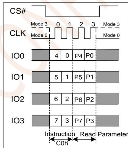
Figure 7.56 Set Read Parameters Instruction (QPI Mode only)
