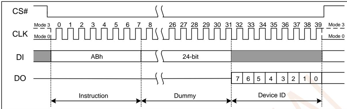
Figure 7.41b Release Power-down / Device ID(SPI Mode)
