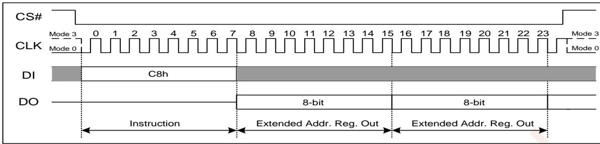
Figure 7.6a Read Extended Address Register Instruction (SPI Mode)
