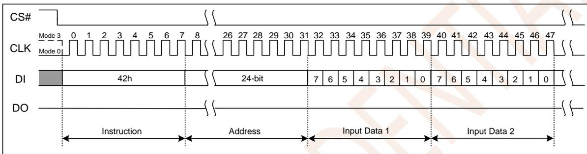
Figure 7.46 Program Security Registers Instruction (SPI Mode only)
