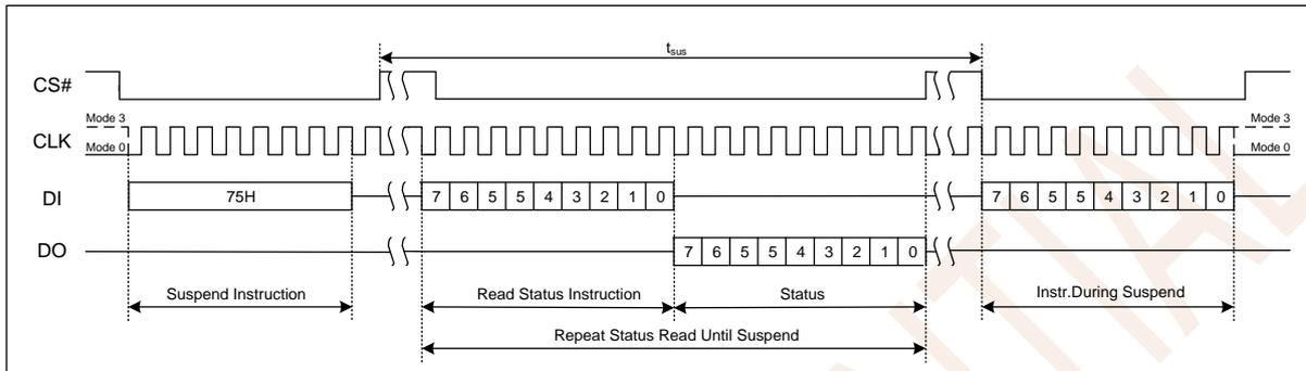
Figure 7.19a Erase / Program Suspend Instruction (SPI Mode)
