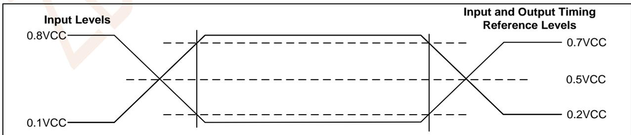
Figure 8.3 AC Measurement I/O Waveform
