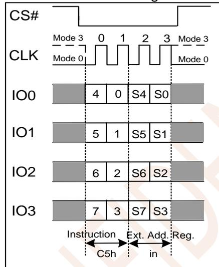
**Figure 7.7b Write Extended Address Register Instruction (QPI Mode)**
