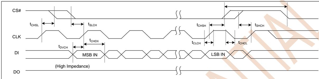
Figure 8.5 Input Timing
