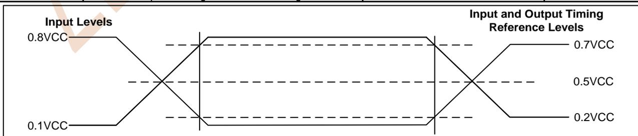
Figure 8.3 AC Measurement I/O Waveform
