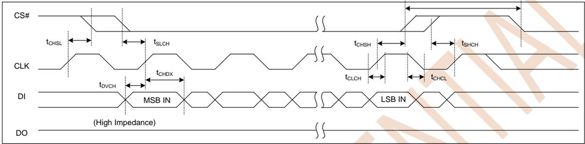
**Figure 8.5 Input Timing**
