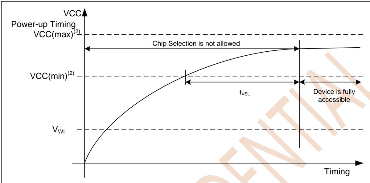
Figure 8.1 Power-up Timing
